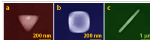
Fig. 1: Scanning electron microscope images of three \text{Cu}_3\text{Si} nanostructures formed on Si substrates of different orientation.
